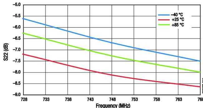
Figure 16. Output Return Loss vs Frequency Across Temperature (Small Signal, P<sub>IN</sub> = -20 dBm)
