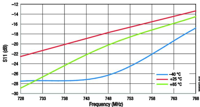
Figure 15. Input Return Loss vs Frequency Across Temperature (Small Signal, P<sub>IN</sub> = -20 dBm)
