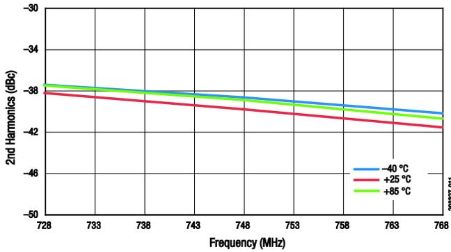
Figure 11. 2<sup>nd</sup> Harmonic vs Frequency Across Temperature @ Pout = +28 dBm (CW)
