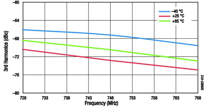
Figure 12. 3<sup>rd</sup> Harmonic vs Frequency Across Temperature @ Pout = +28 dBm(CW)
