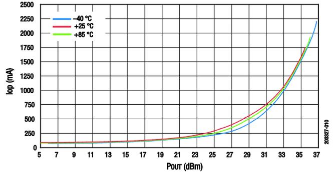
Figure 10. Operating Current vs Pout Across Temperature
